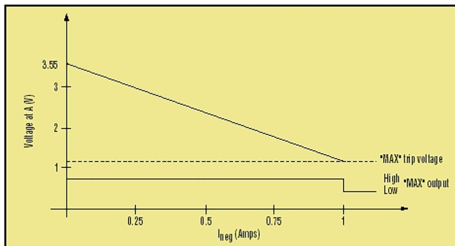
2. The signal voltage "A" in Figure 1 varies with load current as shown, producing the digital warning signal (MAX) at the specified maximum. Polarity of this signal can be easily changed.
