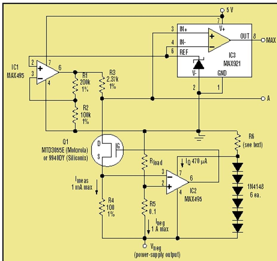
1. This circuit monitors high-side load current into a negative supply, generating a digital alarm (MAX) when the current reaches its maximum.
