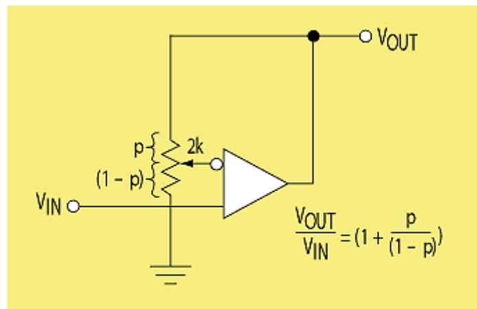
1. A decompensated op amp with the typical gain-set arrangement can exhibit instability when low gain settings are used.
