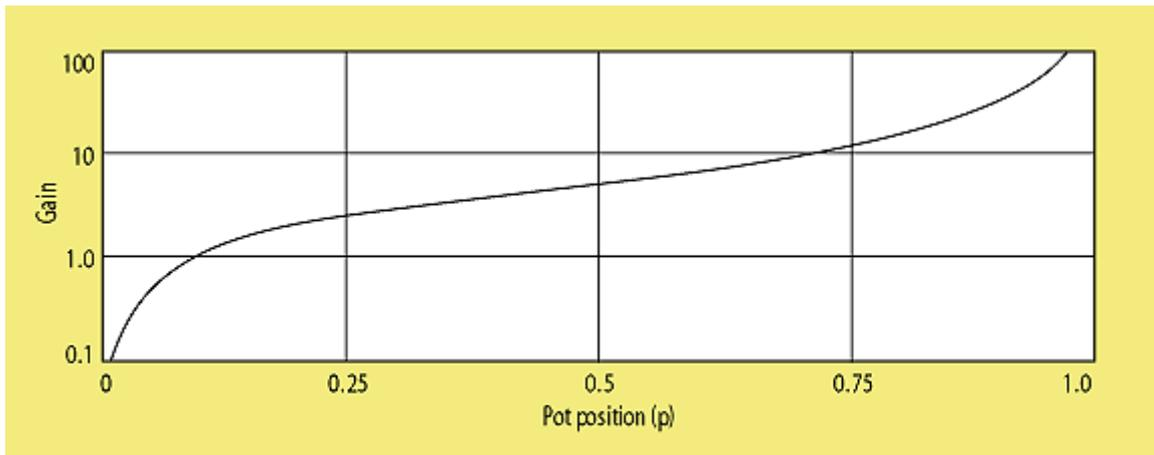
4. The resulting composite gain-versus- $p$  curve ( $G = G_I \times G_O$ ) is shown. The possible gain settings extend from zero (at  $p = 0$ ) to the open-loop gain of the op amp (at  $p = 1$ ).
