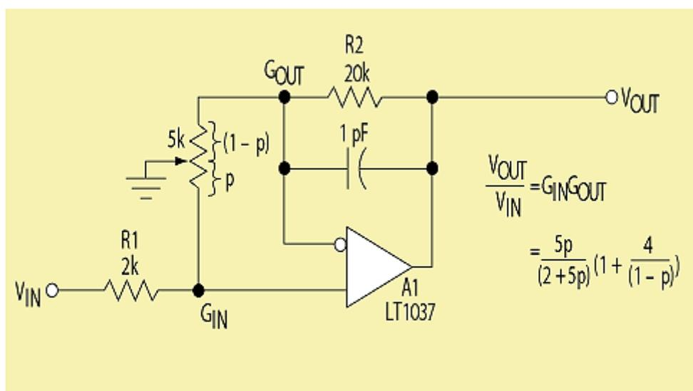
3. By modifying Figure 2b's topology, the input attenuator can be made variable by grounding the pot wiper to create two mechanically linked but electrically independent variable resistors.
