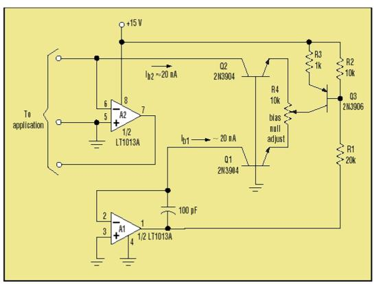
2. Ideal for inverting-amplifier applications, this circuit acts a bias canceller for single-rail op amps, providing the bias-current sink needed by their input networks.
