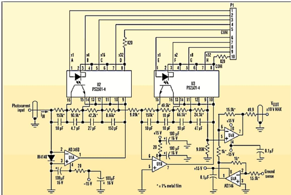
1. This programmable-gain transimpedance amplifier was designed specifically to accommodate the wide dynamic range of sunlight intensity, as well as the demands of low-noise, high-gain, wide-bandwidth signal processing.
