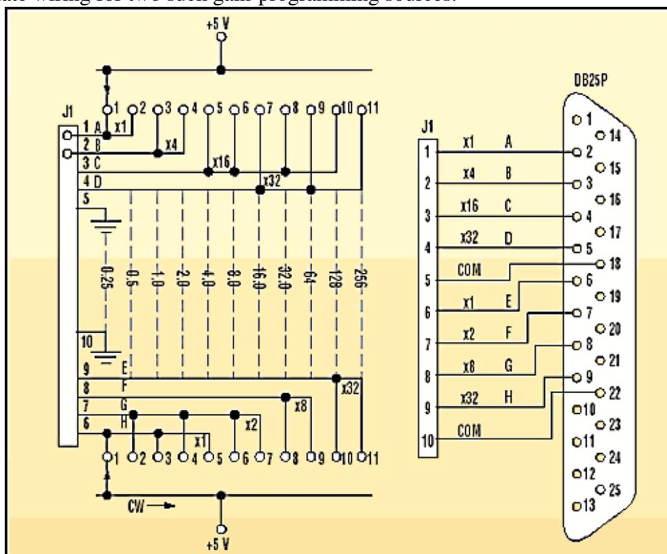
**2.** For control of transimpedance gain, the appropriate wiring for controlling the gain-setting optocouplers for both manual (left) and automated (right) control is shown.
