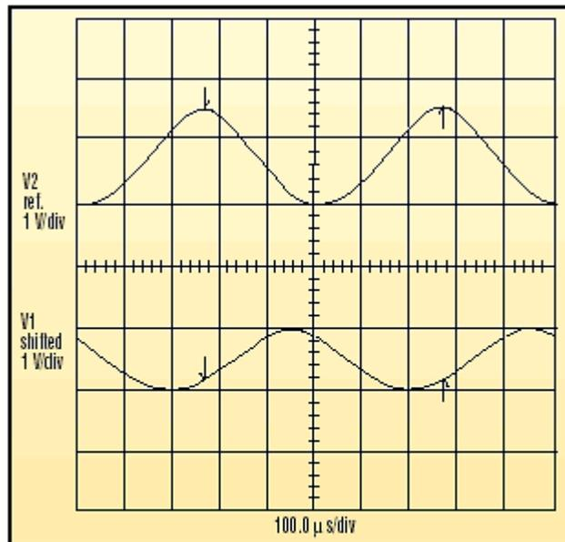
**2. A  $225^\circ$  phase-shift is produced when the DIP switch is set to 160. The amplitude of each sine-wave output can be adjusted using the corresponding potentiometer.**
