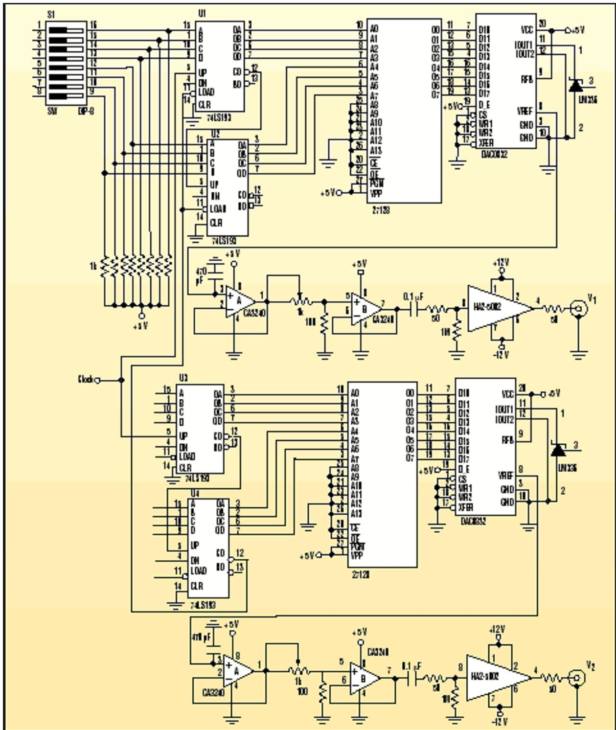
1. This digital waveform generator produces a reference sine-wave output on channel V2 (the reference) and a shifted sine-wave output on channel V1 (with a 0° to 360° phase-shift). The phase shift of the V1 output can be controlled to a resolution of less than 1.5°.
