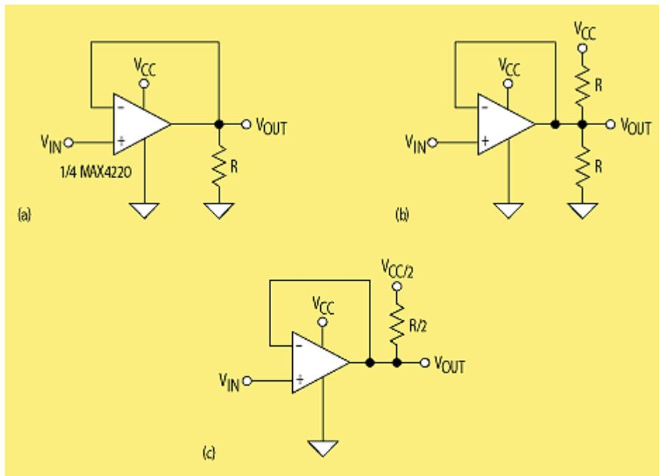
1. The power dissipated in a single-supply op amp biased at mid- $V_{CC}$  (a) is reduced by adding a load-value pull-up to  $V_{CC}$  (b). A Thevenin-equivalent circuit aids analysis (c).
