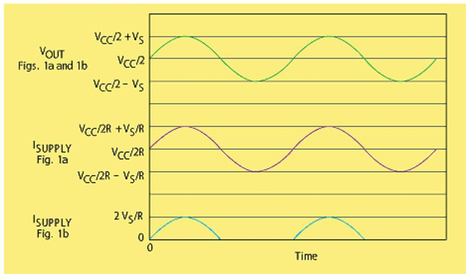
3. These waveforms illustrate the op-amp voltage and current relationships for the circuits shown in Figures 1a and 1b.
