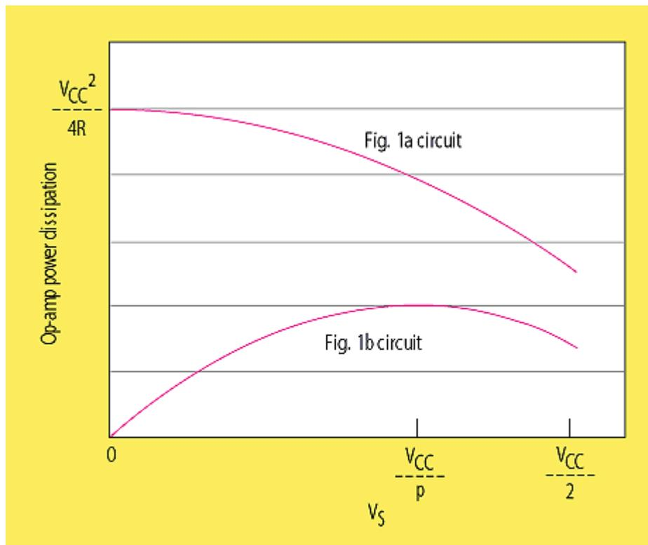
4. The power dissipation in the op amp of Figure 1a is always significantly greater than the dissipation in the op amp of Figure 1b.
