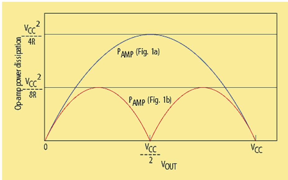
2. The maximum power dissipation, occurring at the quiescent point, of the op amp in Figure 1a is twice that of the op amp in Figure 1b.
