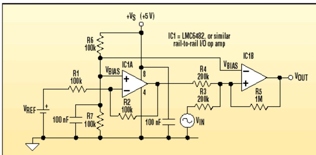
**1.** This single-supply, noninverting Schmitt trigger has symmetrical thresholds around the reference voltage,  $V_{REF}$ . The bias voltage is also dependent only on the values of R6 and R7.
