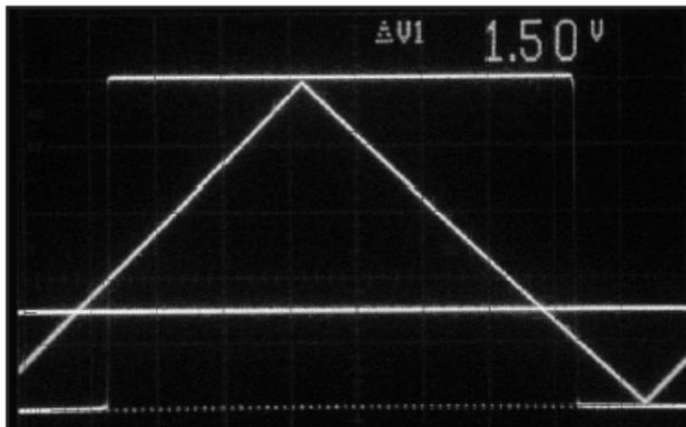
**2.** This scope photo illustrates the circuit's symmetric thresholds and excellent low-frequency performance with  $V_{REF} = 1.5 \text{ V}$ .
