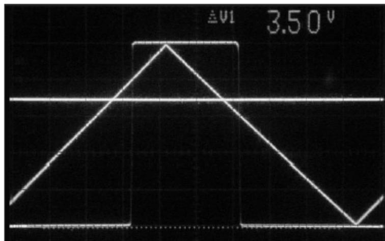
**3.** The thresholds remain symmetrical about  $V_{REF}$  ( $V_{TU} = 4 \text{ V}$  and  $V_{TL} = 3 \text{ V}$ ) even when  $V_{REF}$  has been increased to  $3.5 \text{ V}$ .
